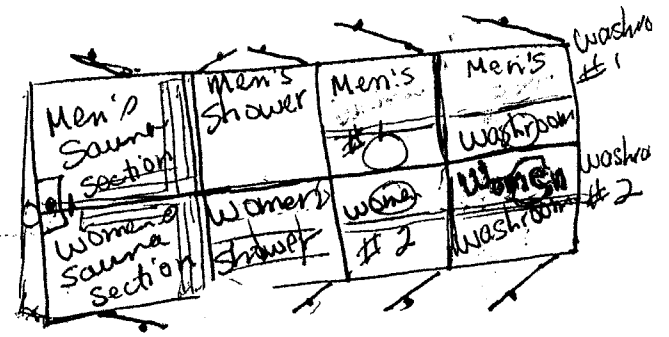
top view of toilets showers & sauna
